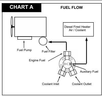
The diesel fired heater fuel outlet port on the TWHF Hot Fox™ is 1/8" female pipe thread. Brass adapters are available from Arctic Fox or local suppliers to connect the fuel supply hose to your diesel fired heater. See Chart D for Arctic Fox part numbers.
